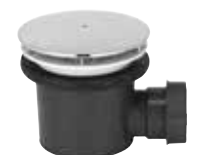
90mm fast flow waste, includes hair trap and chrome cover.
