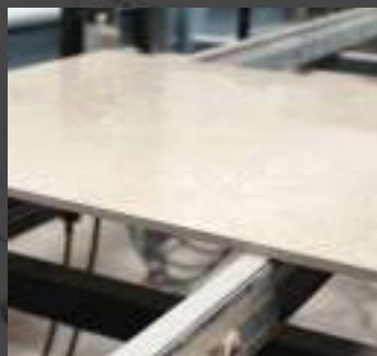
Dry grinding of the tile after the «Easy-to-clean» application treatment. The tile is tested by applying products that can stain traditionally polished products and by determining whether the colour or gloss have suffered after dry cleaning or using a cleaning agent.
