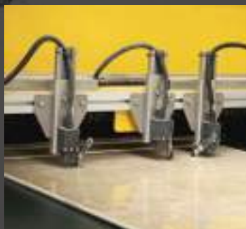
Traditional polish on matt tile before grinding.
